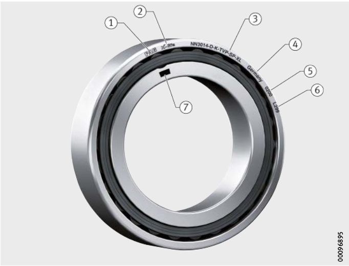
Figure 8 Marking of double row bearings
