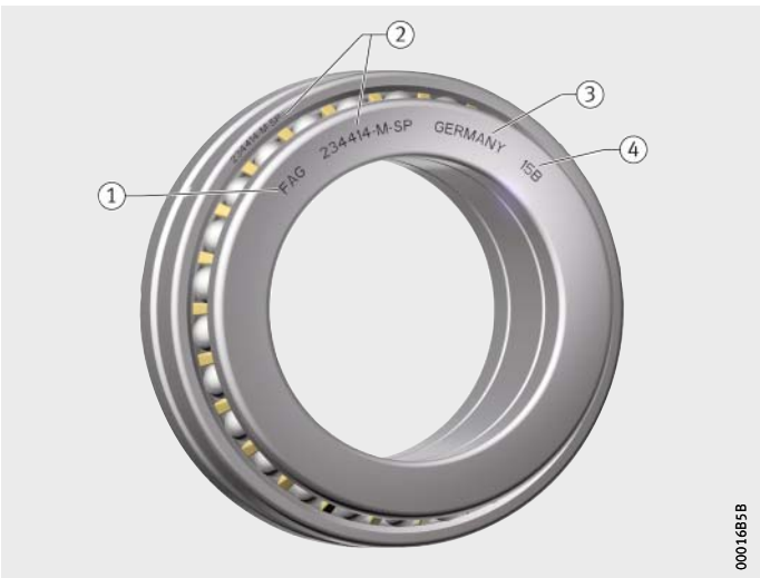
Figure 5 Marking of bearings
