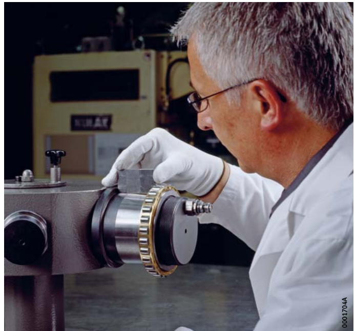
Figure 5 Measuring the spacing from the shaft shoulder
